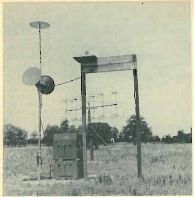
Antennas and equipment cases contain radar-range transponder, central timing recorder and aircraft tracking units.
