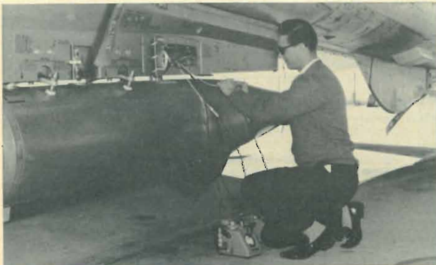
Technician performs final checkout of equipment pod slung beneath fuselage of Air Force F-105 jet fighter prior to low-level simulated mission. Pod contains telemetry gear.
