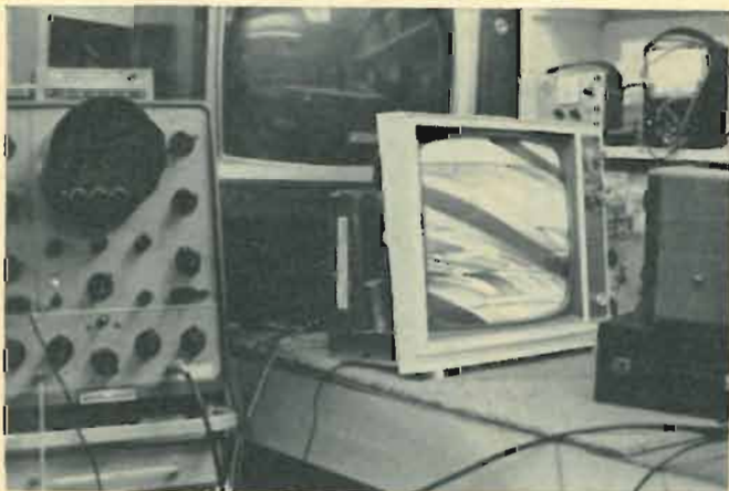
Camera head at right views screen symptom of faulty TV set. Waveshape across bad component is shown on scope.
